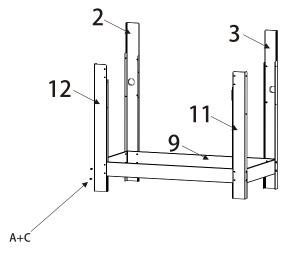
Hardware required: A, M6x12mm, x16, C, M6 Nut, x16
