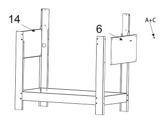
Hardware required: A, M6x12mm, x8, C, M6 Nut. x8
