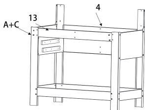
Hardware required: A, M6x12mm, x8, C, M6 Nut, x8
