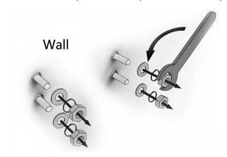
Step3:Installer the heater on the wall
