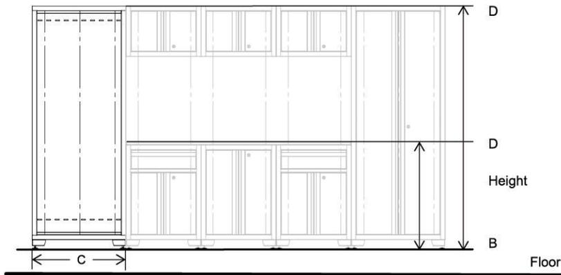
**Note:** Make sure that there are two studs to mount the locker on as it is easiest to start the installation with the locker first. Due to the spacing of the wall studs, some wall cabinets maybe have only one stud to attach to; this is acceptable if the wall cabinets are bolted together.
