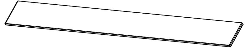
Carefully place the worktop on the cabinets and fasten it with cordless power drill and four screws in the parts package of each base cabinet / 1-drawer cabinet.
