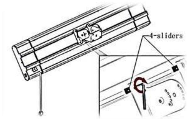
**Step 3:** Fix the part 1 ①,1 on the wall, tighten the four nuts (a part of explosive bolt M6\*50) ①,2 with M6 spanner ①,9
