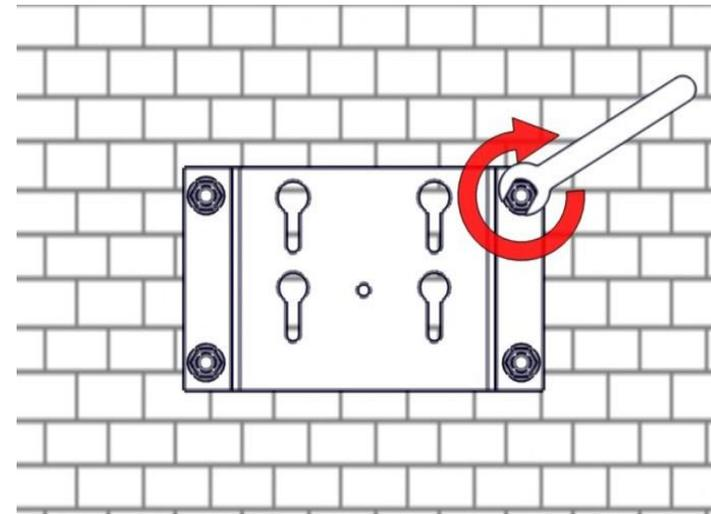
**Step 4:** Put the heater on the wall, slide it into the part 1 ①,1.
