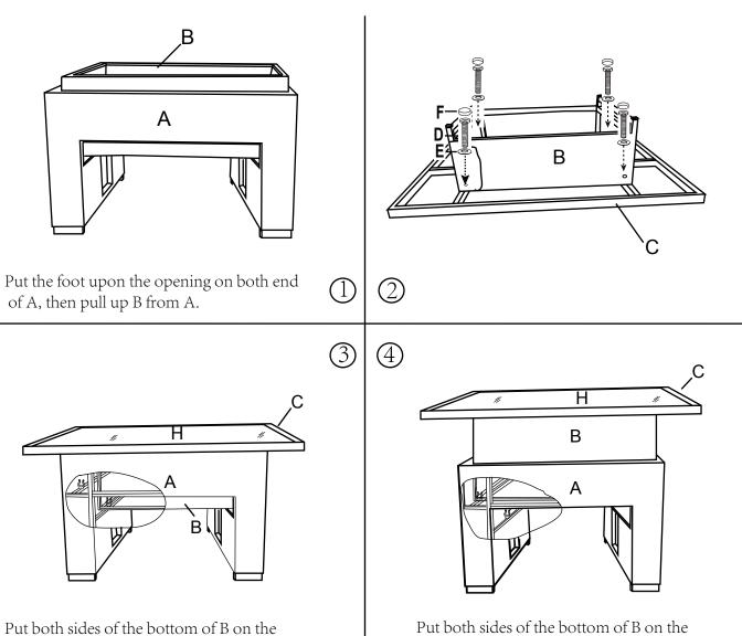
Put both sides of the bottom of B c point of 'U' clips that at the top of
