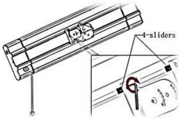
**Step 3:** Fix the part 1 ○,1 on the wall, tighten the four nuts (a part of explosive bolt M6\*50) ○,2 with M6 spanner ○,9
