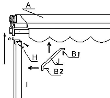
1. Using M8X60(H)screws, assemble the (A) and (I).
