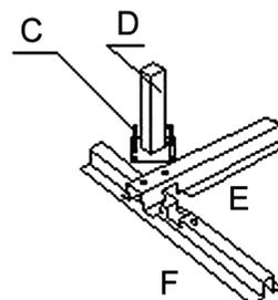
3. Using M8x20(C)screws, assemble the(D),(E)and(F).
