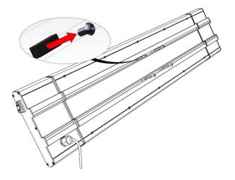
Do not tighten the four M6\*10 screws ③, reserve 2-3mm of gap for step 4.
