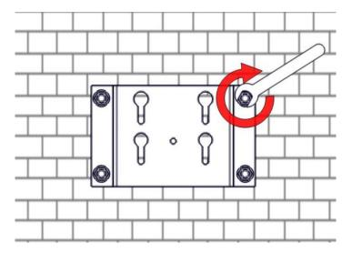
**Step 4:** Put the heater on the wall, slide it into the part 1  $\bigcirc$ , 1.
