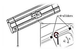
**Step 3:** Fix the part 1  $\bigcirc$ ,1 on the wall, tighten the four nuts (a part of
