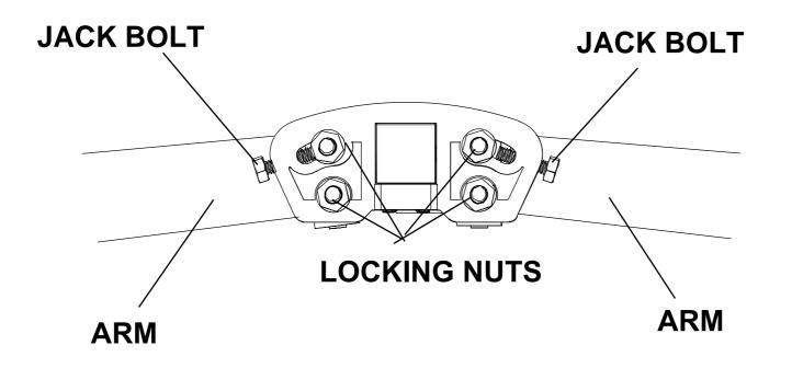
Loosen the locking nuts.
