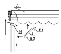
1.Using M8X60(H)screws,assemble the (A) and (I).
