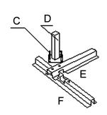
3.Using M8x20(C)screws,assemble the(D),(E)and(F).
